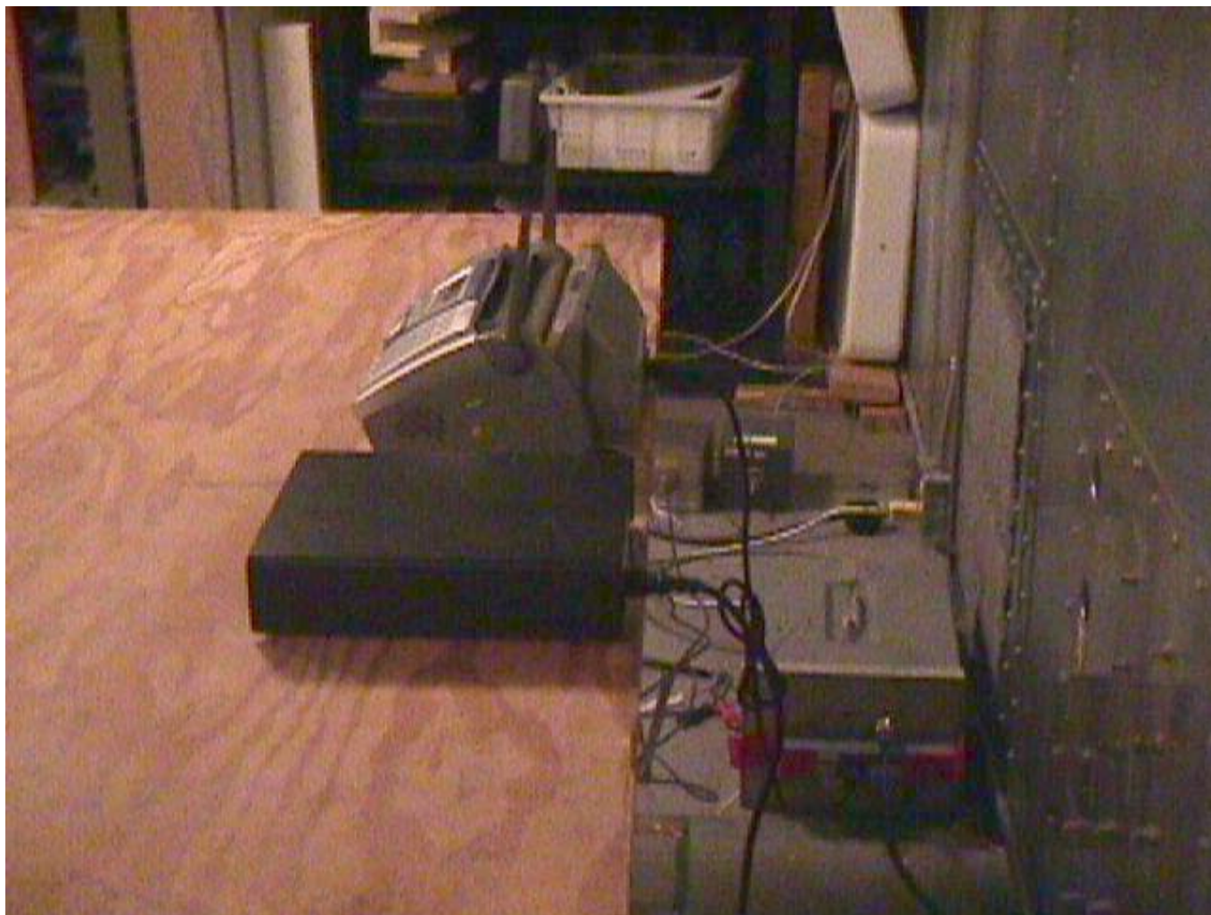
AC Power Line Conducted Emissions (Side View)
