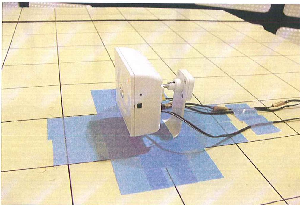
Photograph 5: Set-up for Radiated Emission, EUT Configuration Y-axis
