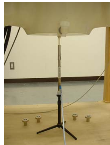
5100-5800MHz System performance check setup
