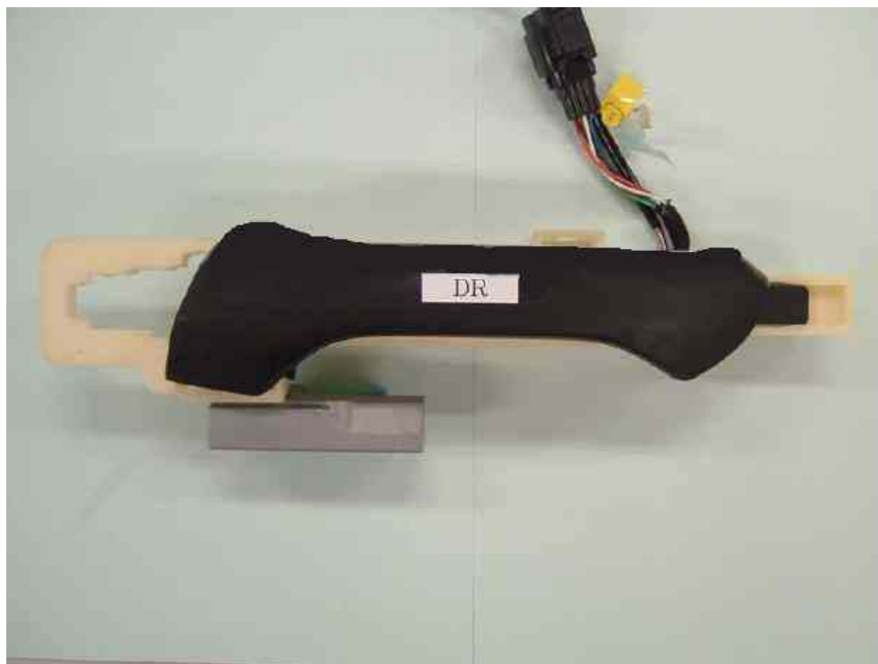
Antenna (Door) Front
