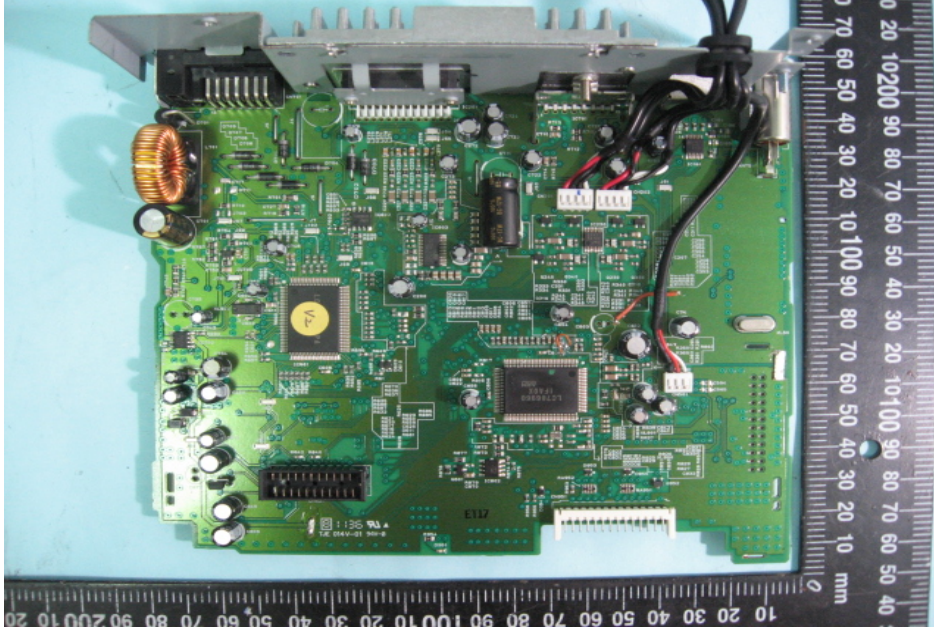
14. Component View of Car Radio PCB
