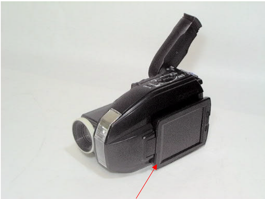
Color LCD electronic view finder (Part of video camera)
