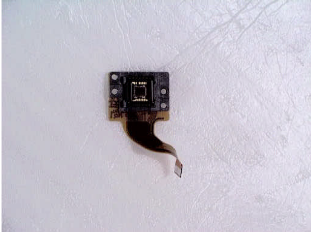
CCD PCB (Top View)
