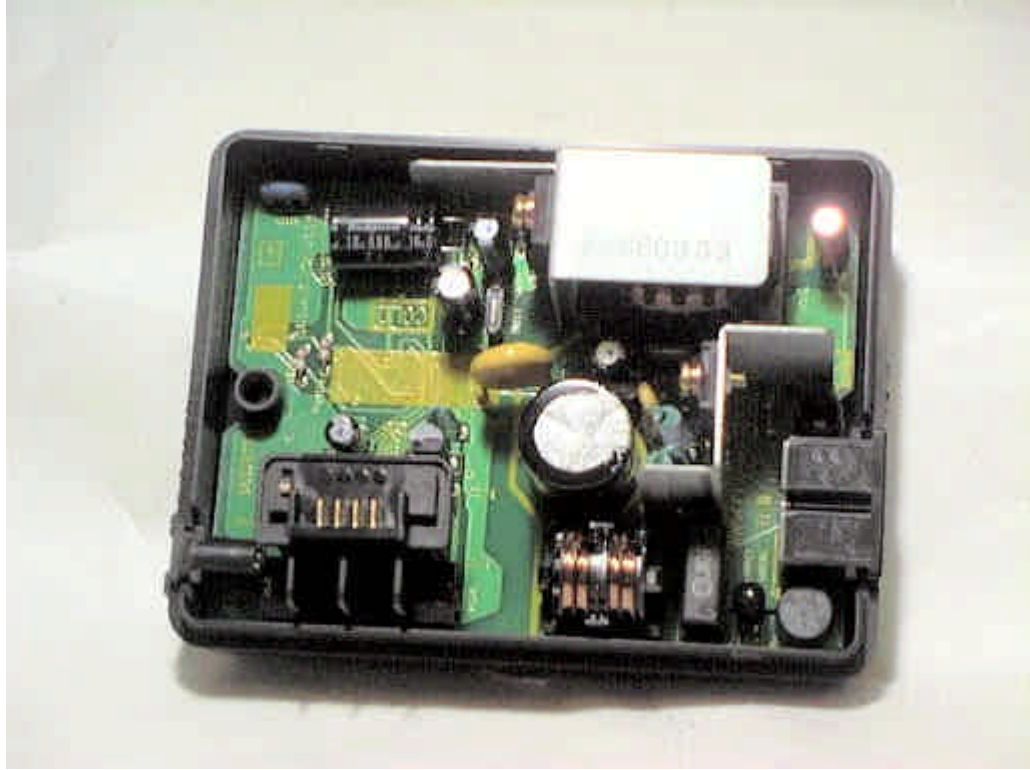
AC Adaptor PCB (Top view)
