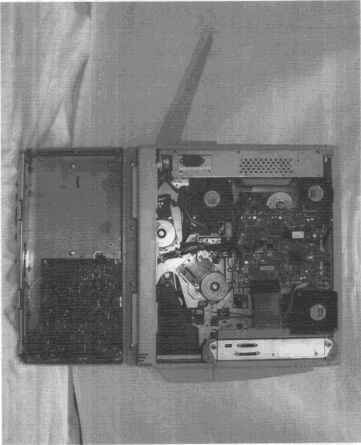
Photo 3 Rear Inside view of Color Laser Printer with Rear Cabinet and Engine Board Cover Removed.
