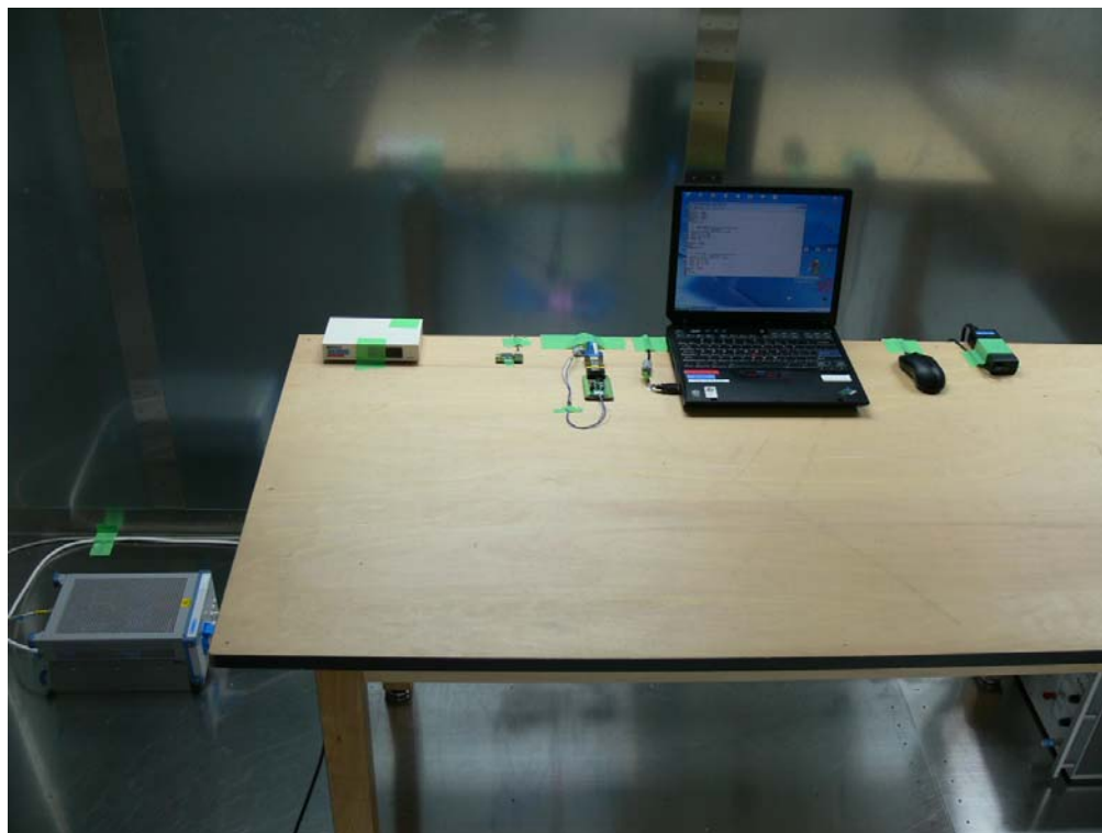
Photograph 2: Set-up for Front View Conducted Testing
