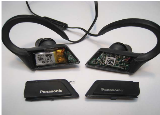
Left side (Battery and Thermistor board)
