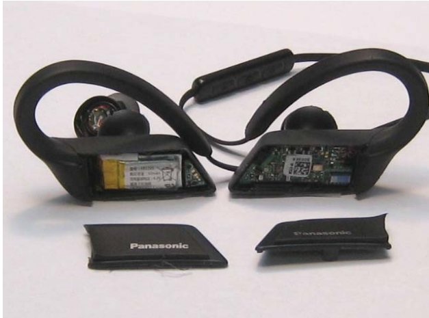
Left side (Battery and Thermistor board)
