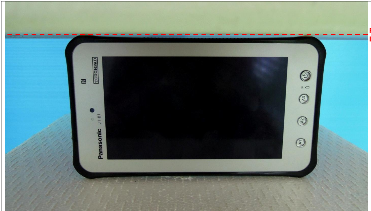
SAR Test Position : EDGE2 with 0 mm Gap
