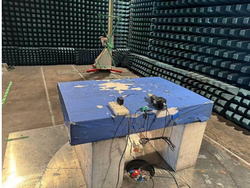
Test setup photo for radiated emission test (30MHz-1GHz)
