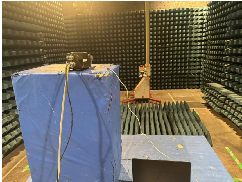
Test setup photo for radiated emission test (Above 1GHz)
