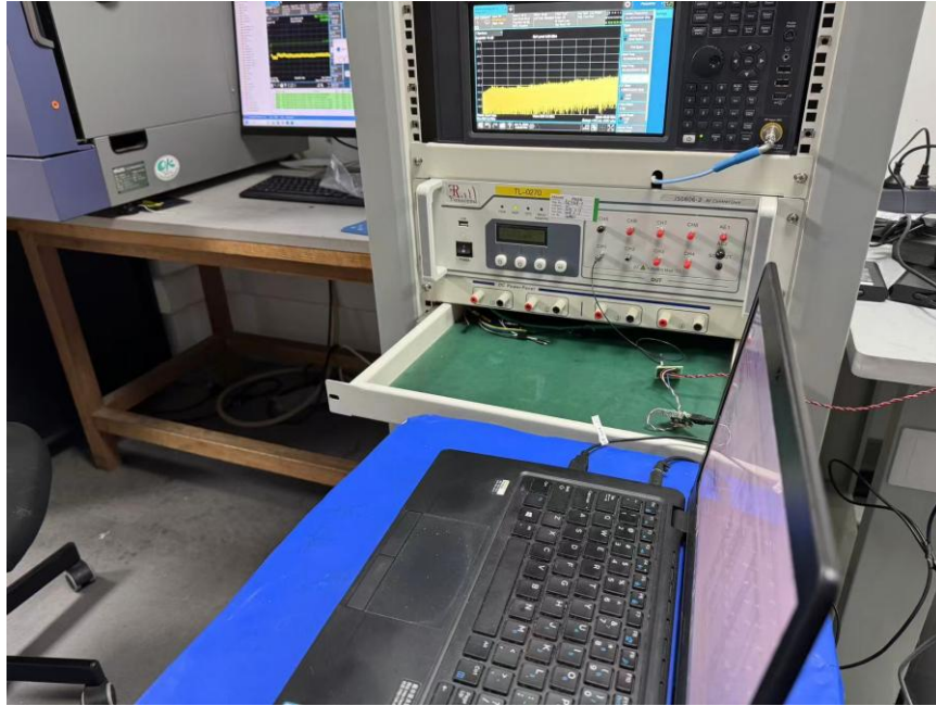
Test setup photo for Conducted RF test
