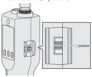
Turn OFF the power switch of the power adapter, or disconnect the power plug from the outlet.
