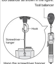
Hang the screwdriver hanger on a hook of the tool balancer.
