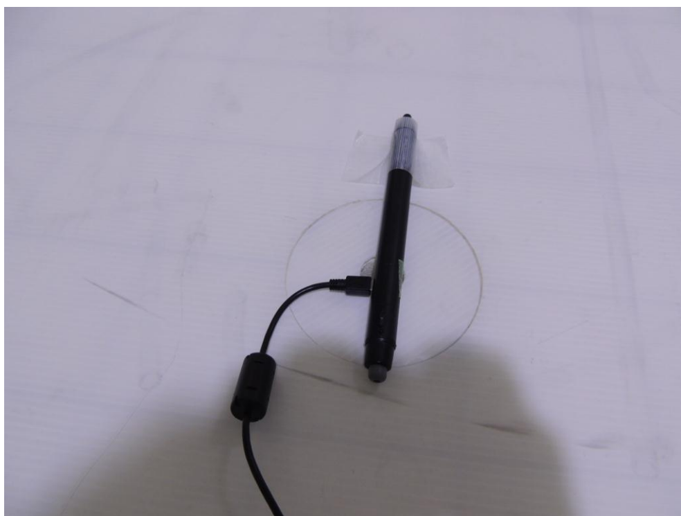
Photograph 4: Set-up for Radiated Emission, EUT Configuration X-Axis
