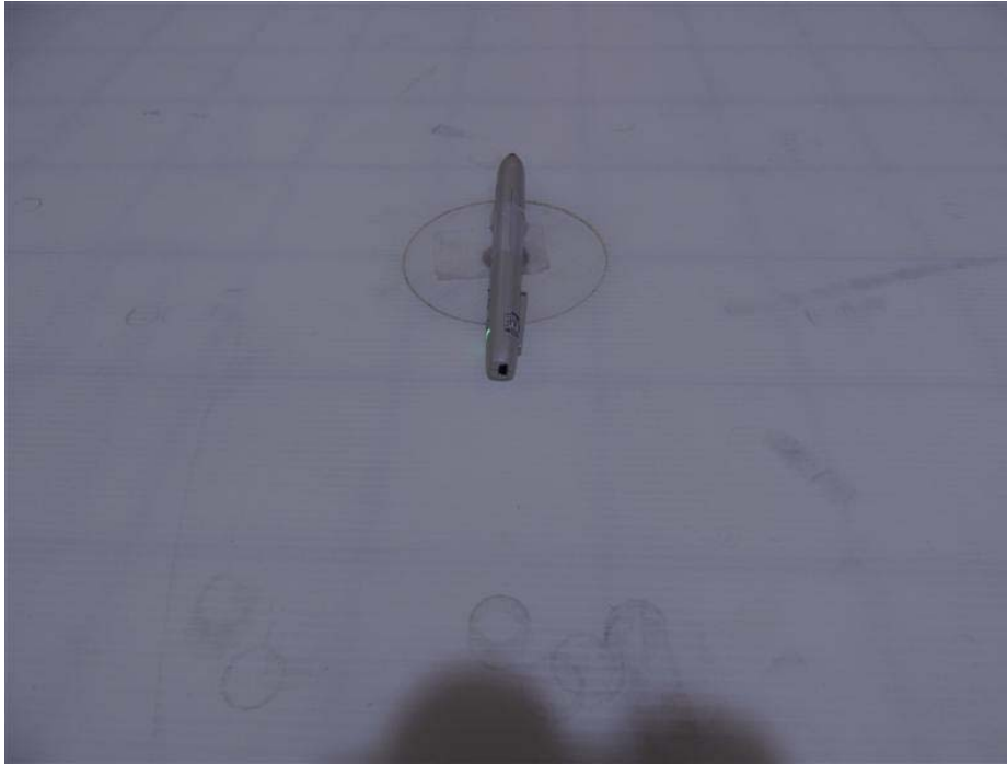
Photograph 4: Set-up for Radiated Emission, EUT Configuration Y-Axis
