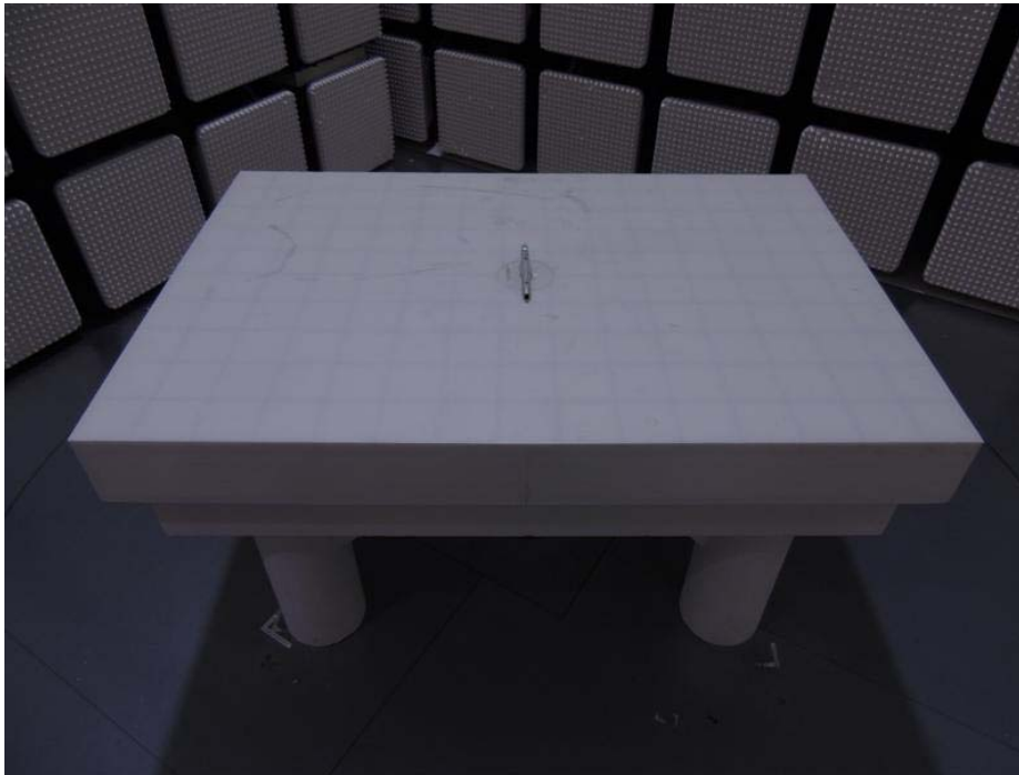
Photograph 2: Set-up for Radiated Emission of Transmitter
