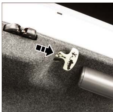
Internal Emergency Trunk Release
