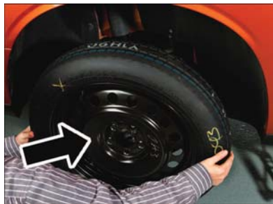
Installing Compact Spare
