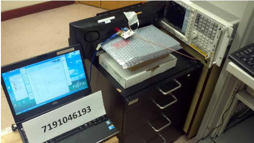
Average Frequency Dwell Time Test Setup
