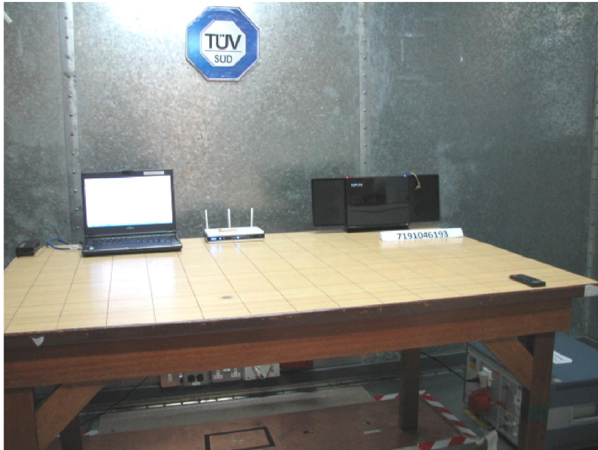
Conducted Emissions Test Setup (Front View)
