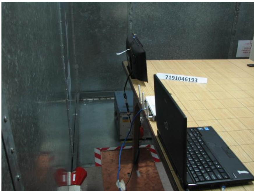
Conducted Emissions Test Setup (Rear View)
