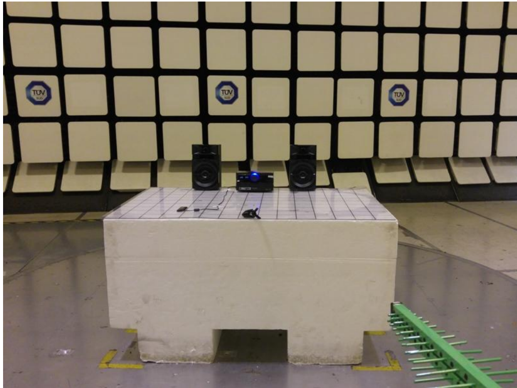
Radiated Emissions Test Setup (Front View)
