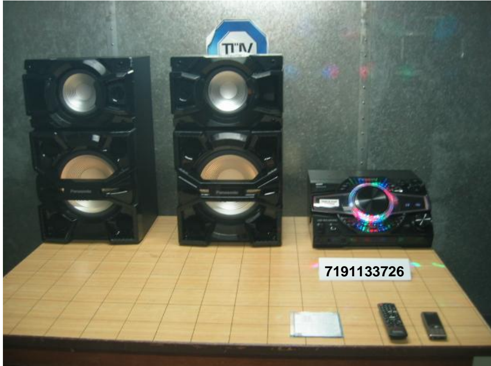
Conducted Emissions Test Setup (Front View)
