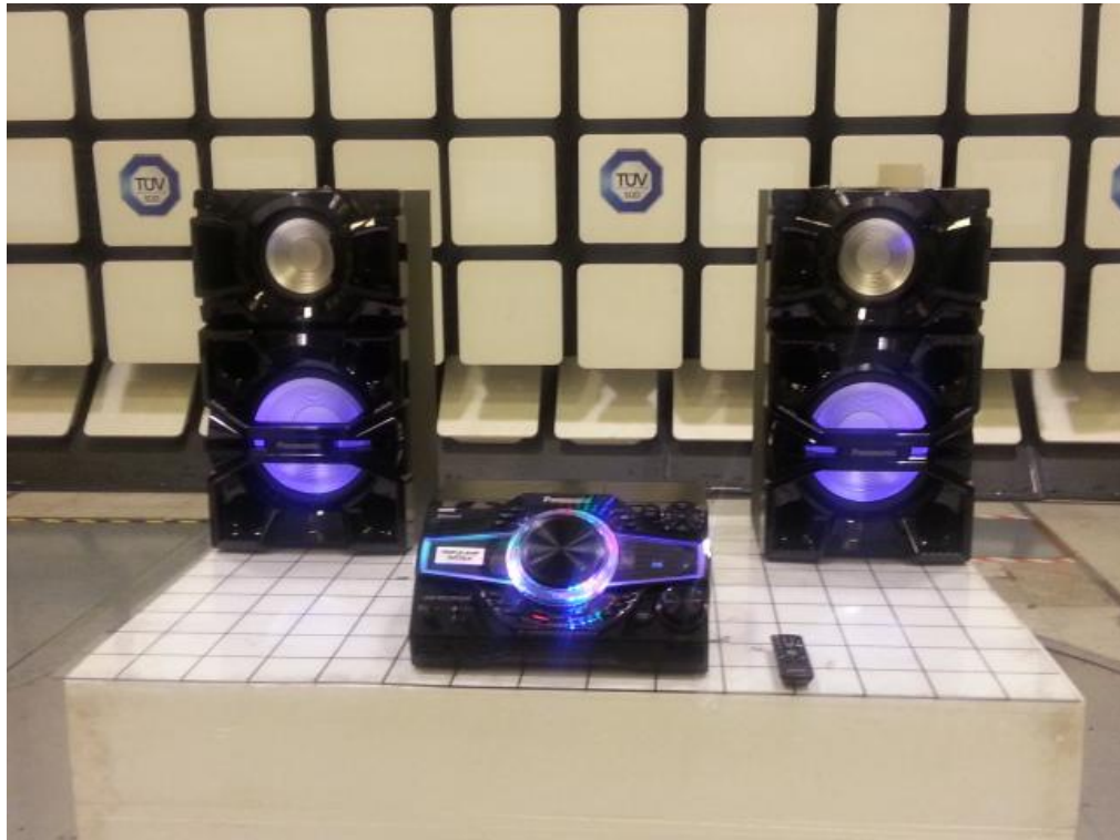
Radiated Emissions Test Setup (Front View)
