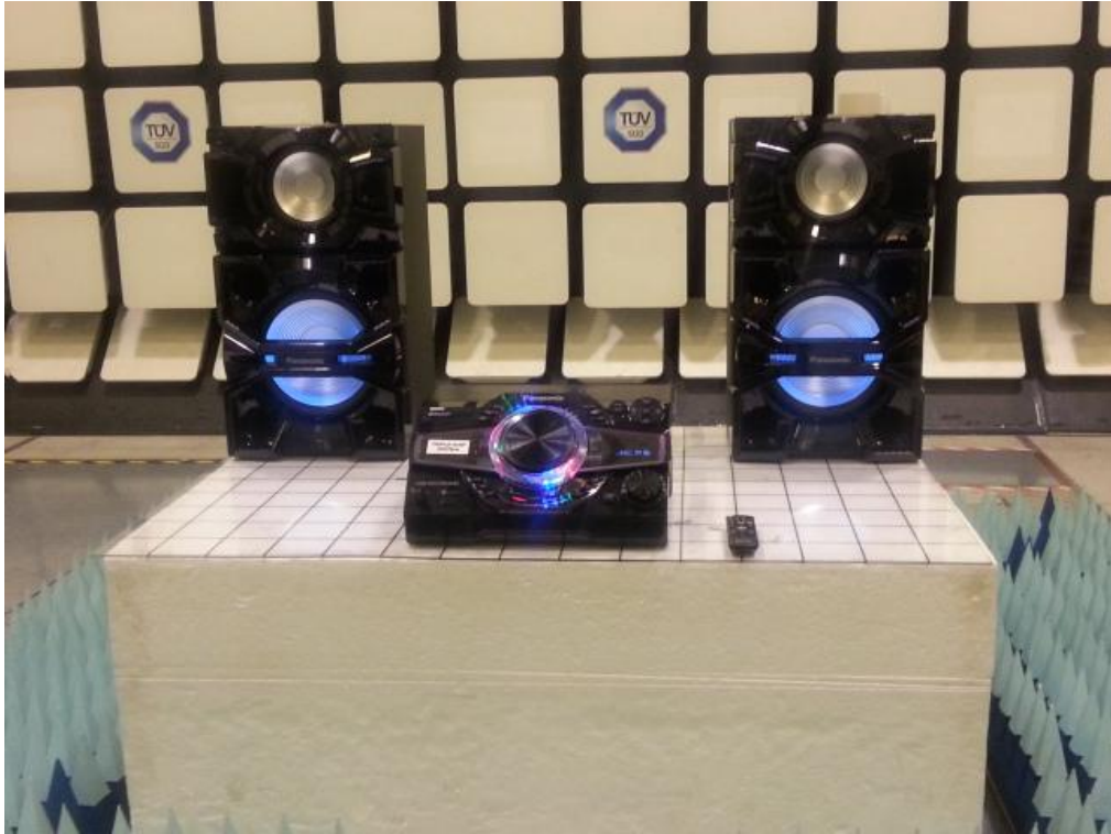
Radiated Emissions Test Setup (Front View)
