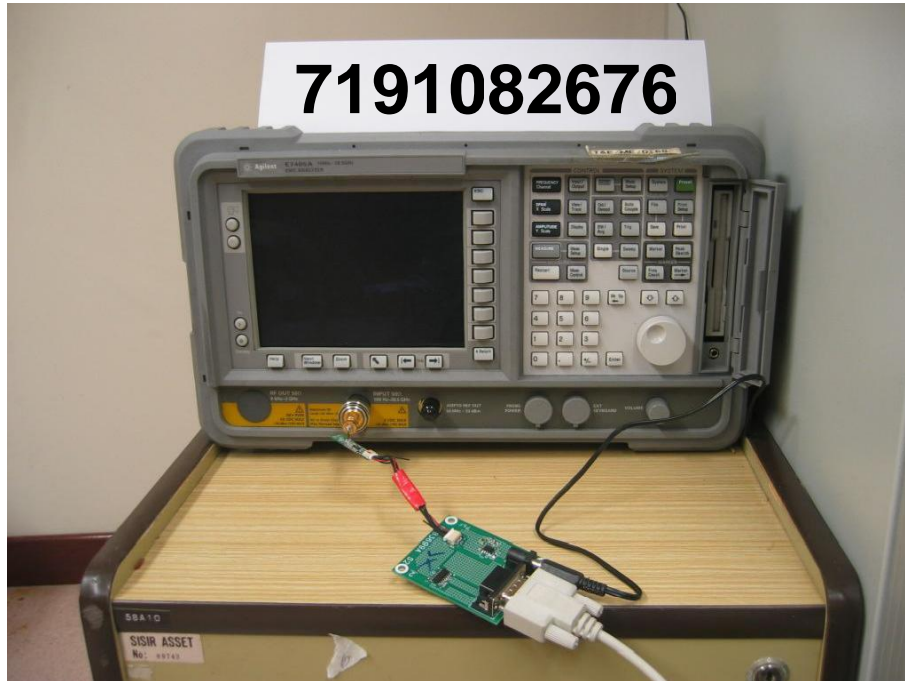
Carrier Frequency Separation Test Setup
