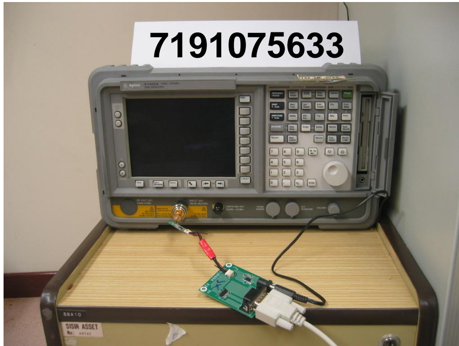
Average Frequency Dwell Time Test Setup
