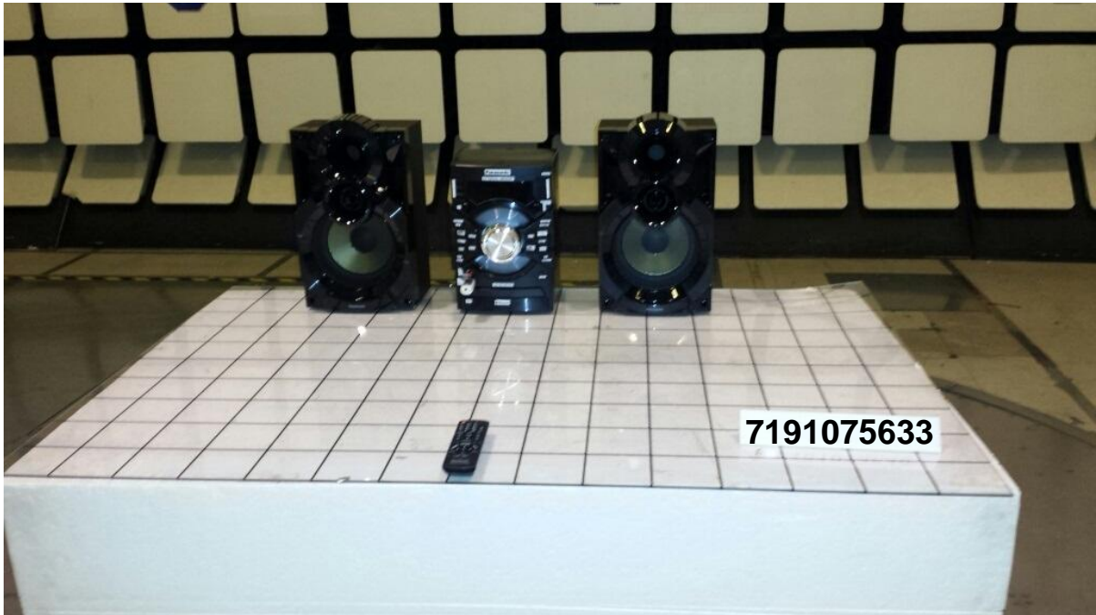
Radiated Emissions Test Setup (Front View)
