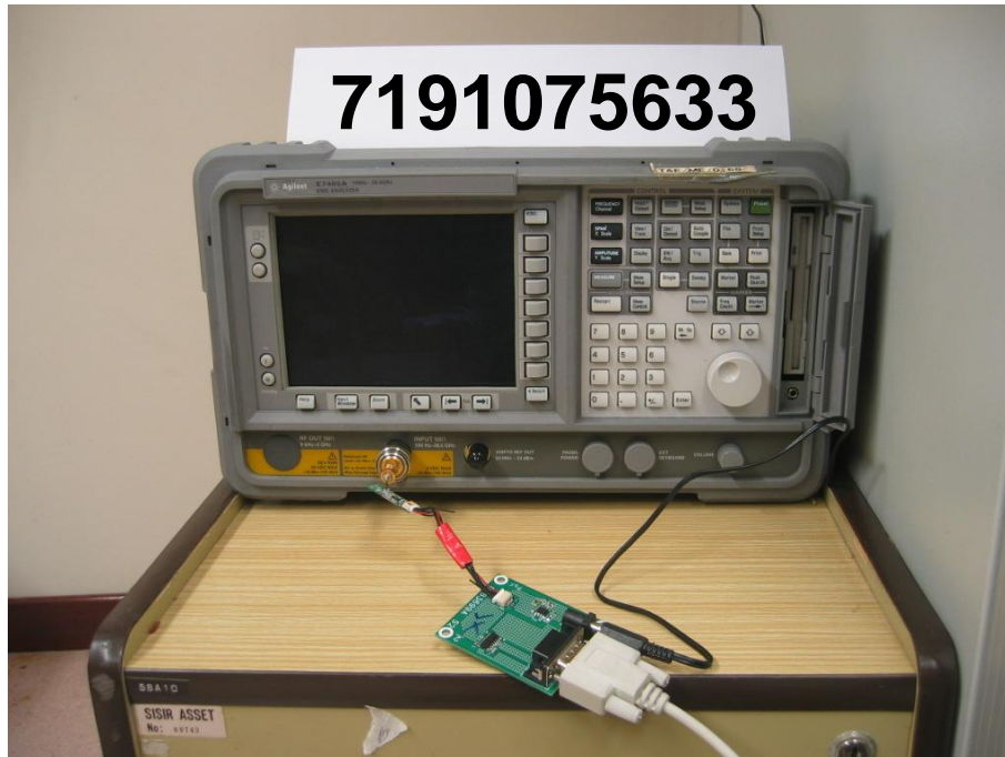
Spectrum Bandwidth (20dB Bandwidth Measurement) Test Setup
