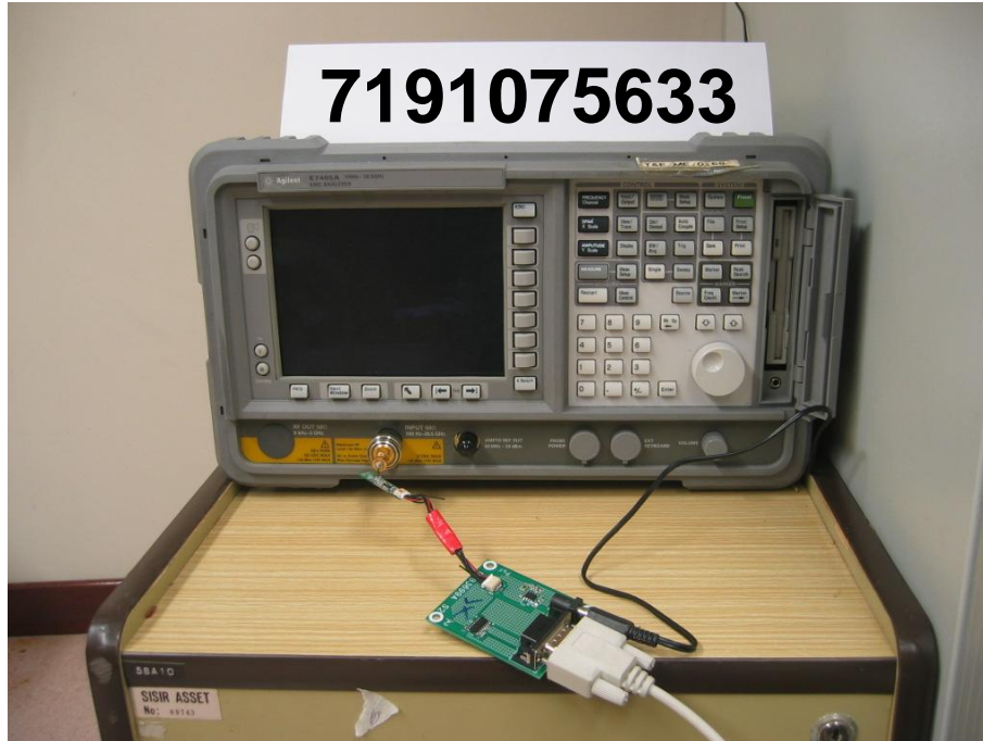
RF Conducted Spurious Emissions Test Setup
