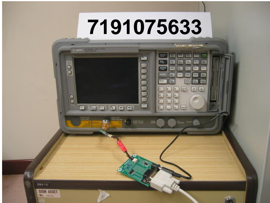
Number of Hopping Frequencies Test Setup
