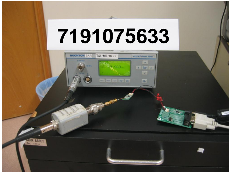
Maximum Peak Power Test Setup
