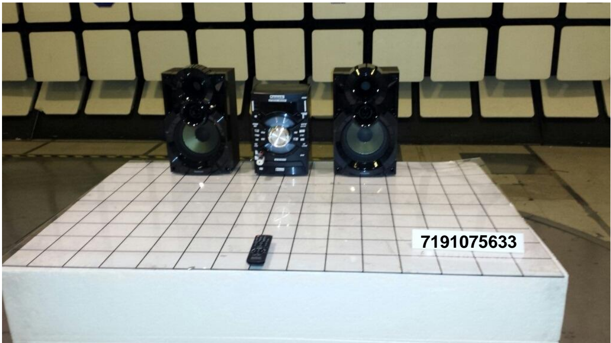
Radiated Emissions Test Setup (Front View)
