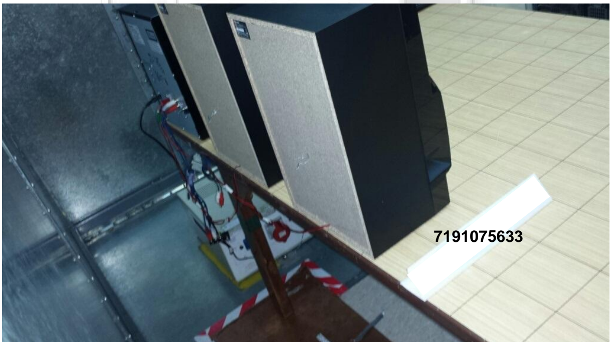
Conducted Emissions Test Setup (Rear View)
