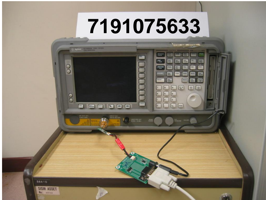
Peak Power Spectral Density Test Setup
