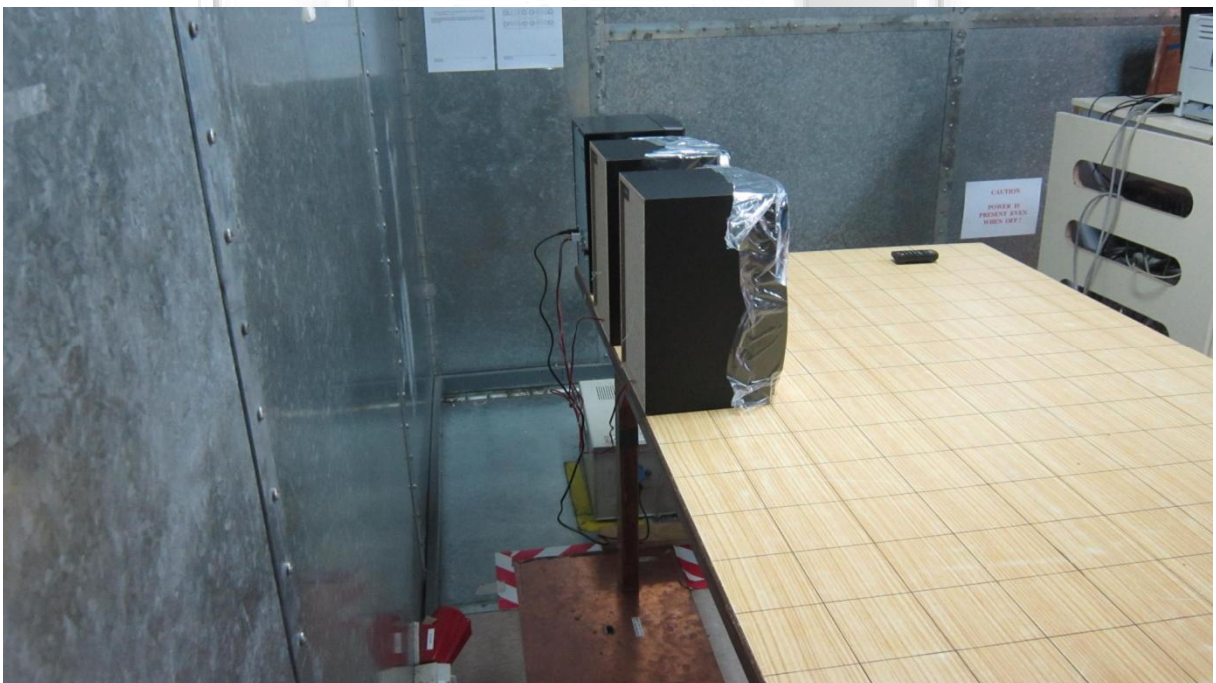
Conducted Emissions Test Setup (Rear View)
