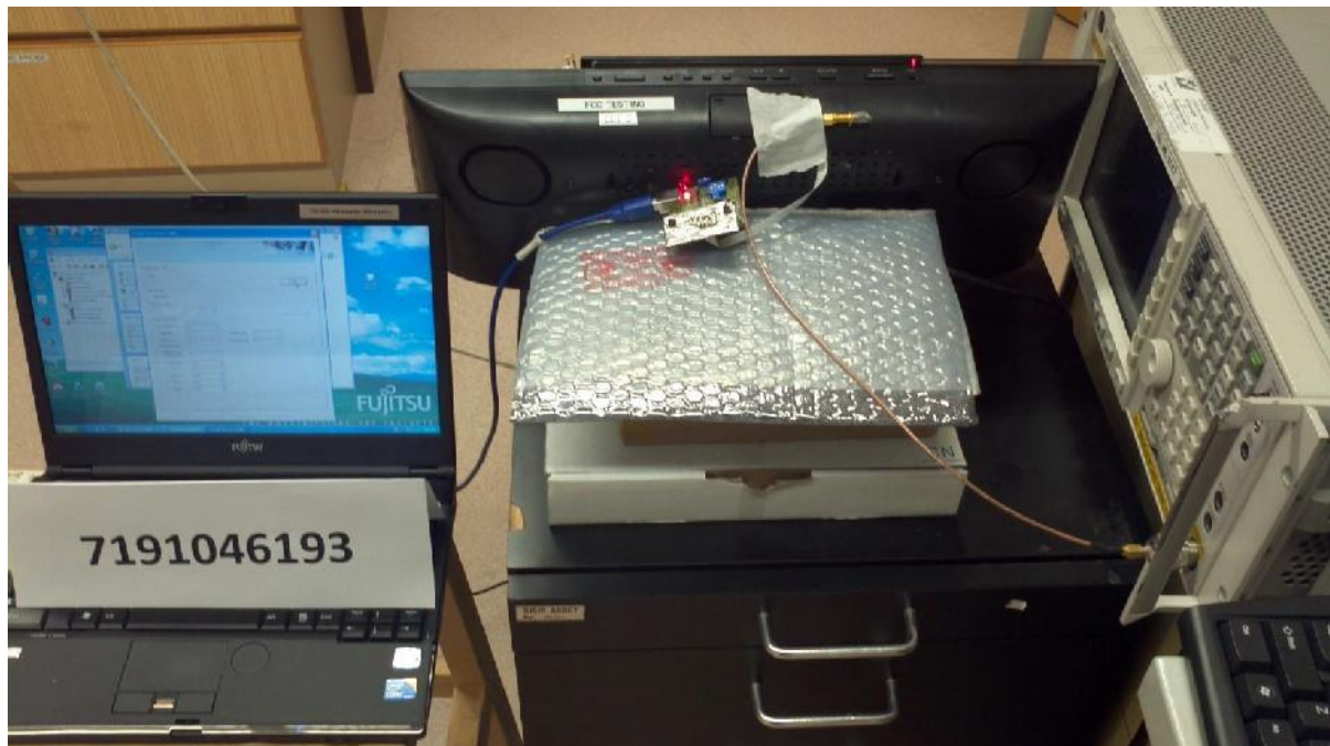
Number of Hopping Frequencies Test Setup
