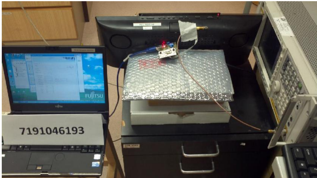
Carrier Frequency Separation Test Setup
