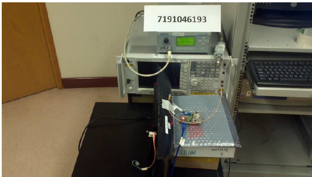
Maximum Peak Power Test Setup
