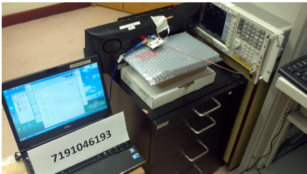
Spectrum Bandwidth (20dB Bandwidth Measurement) Test Setup
