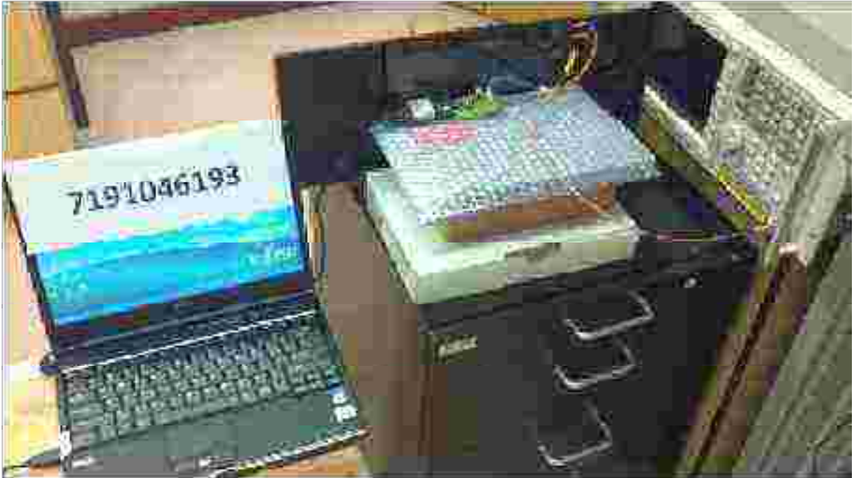
Spectrum Bandwidth (6dB Bandwidth Measurement) Test Setup
