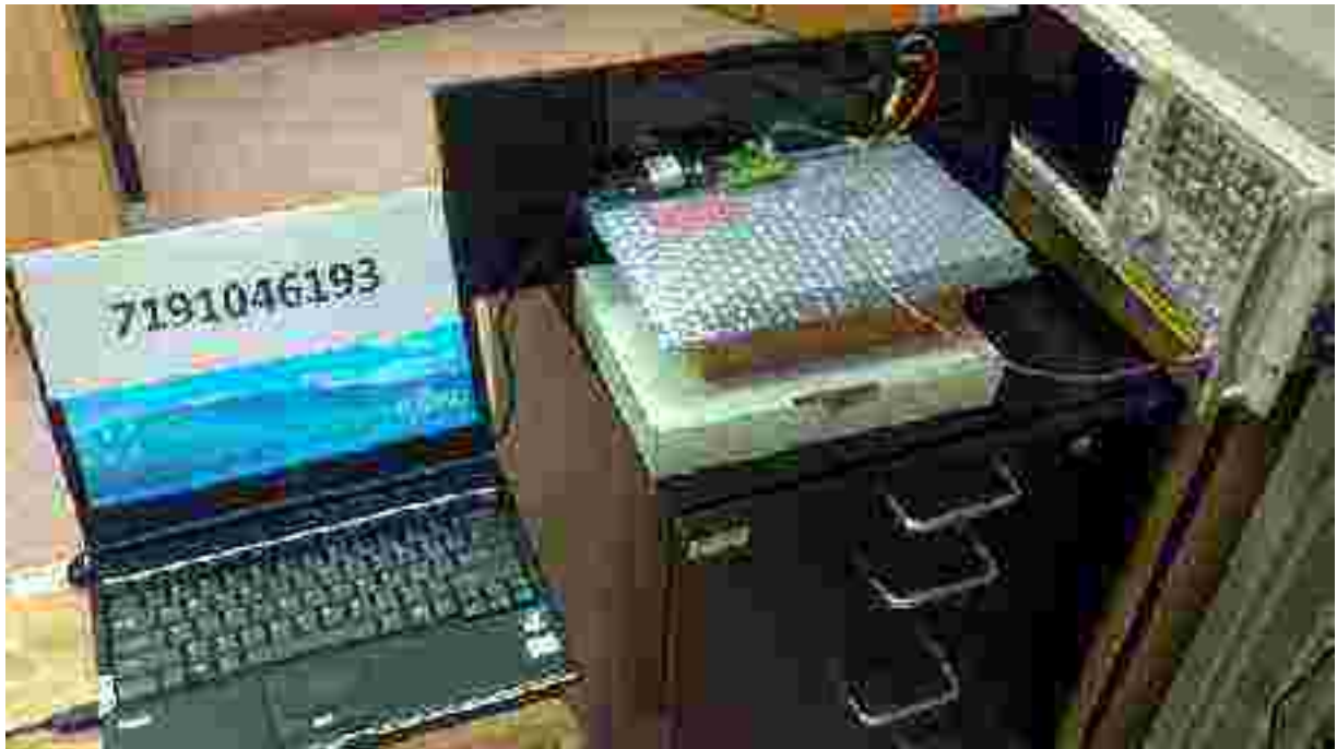
Peak Power Spectral Density Test Setup
