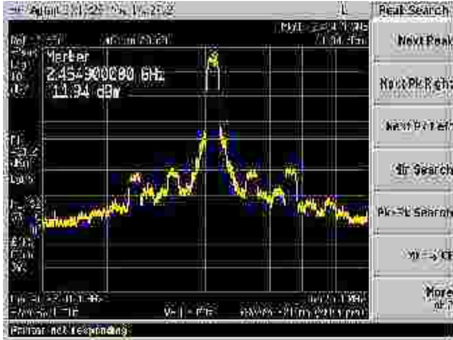
Plot 307 – Channel 11 (upper ch) @ QPSK 18Mbps
