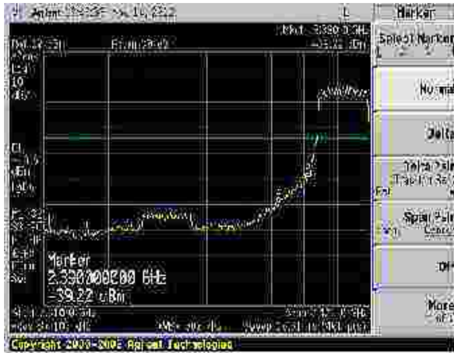
Plot 553 – Lower Band Edge at 2.4000GHz @ QPSK18Mbps
