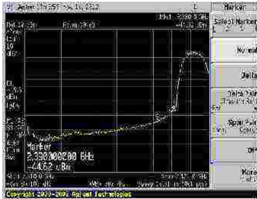
Plot 551 – Lower Band Edge at 2.4000GHz @ CCK 11Mbps
