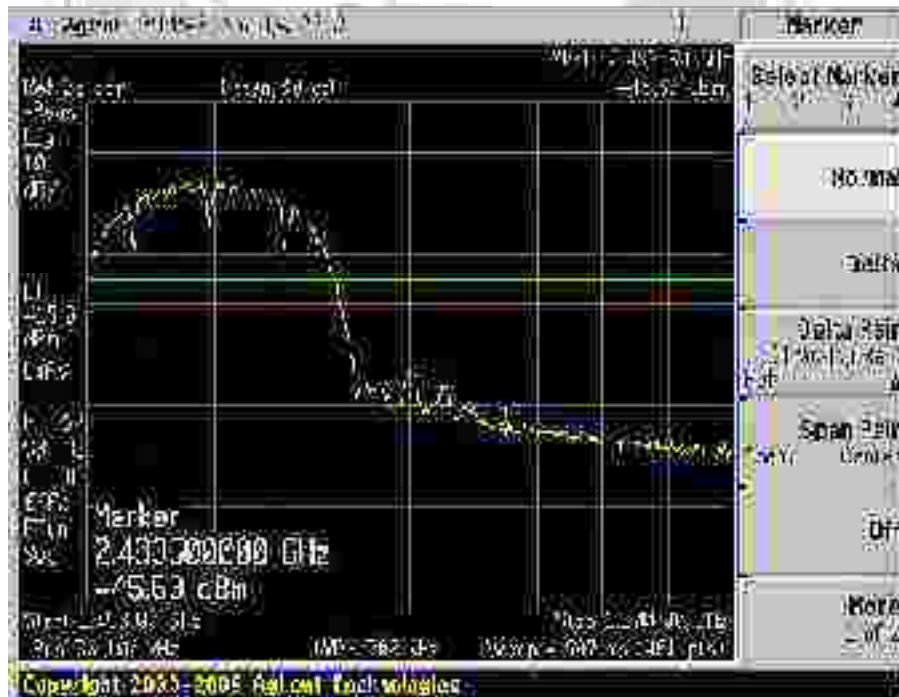
Plot 571 – Upper Band Edge at 2.4835GHz @ DQPSK 2Mbps
