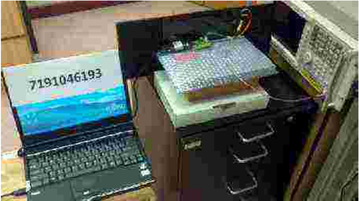
Band Edge Compliance (Conducted) Test Setup
