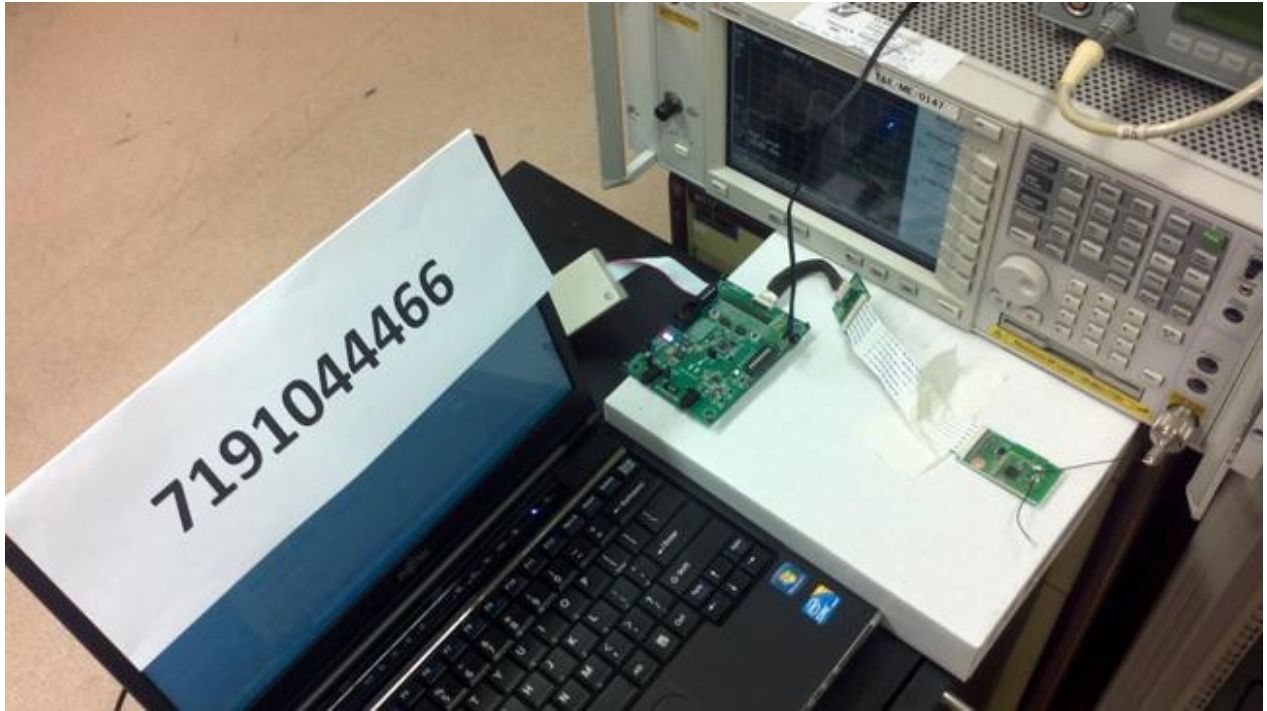
Peak Power Spectral Density Test Setup
