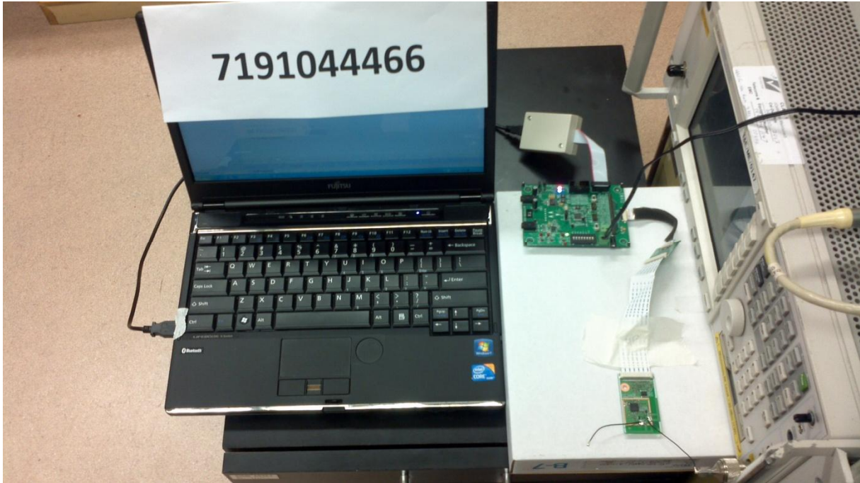
RF Conducted Spurious Emissions (Non-Restricted Bands) Test Setup
