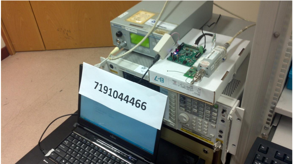
Maximum Peak Power Test Setup
