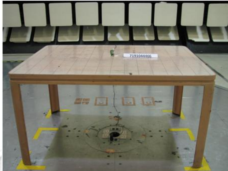
Radiated Emissions Test Setup (Front View)
