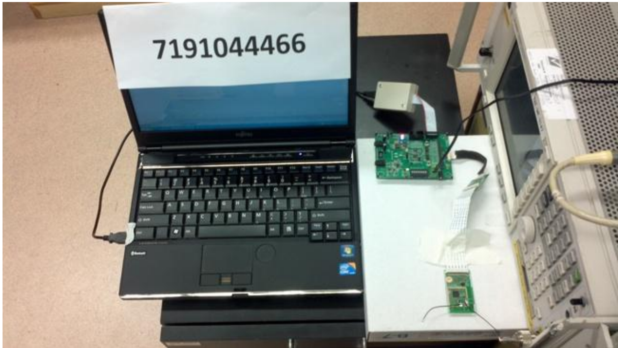
Band Edge Compliance (Conducted) Test Setup
