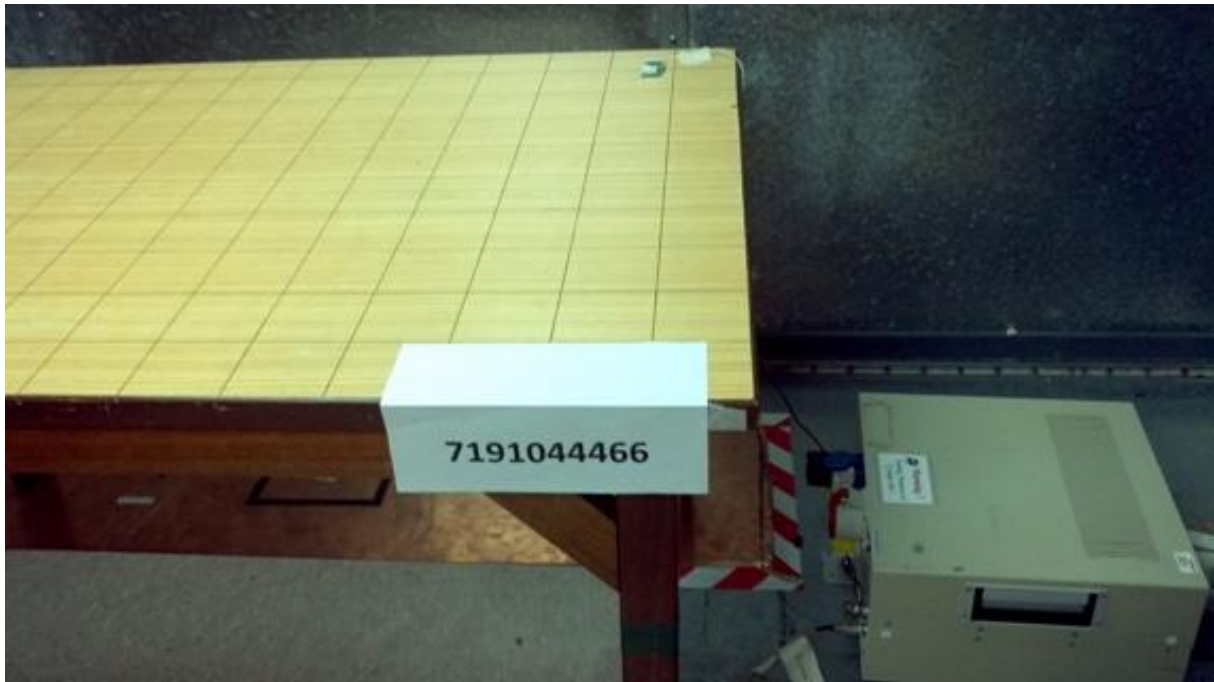
Conducted Emissions Test Setup (Front View)
