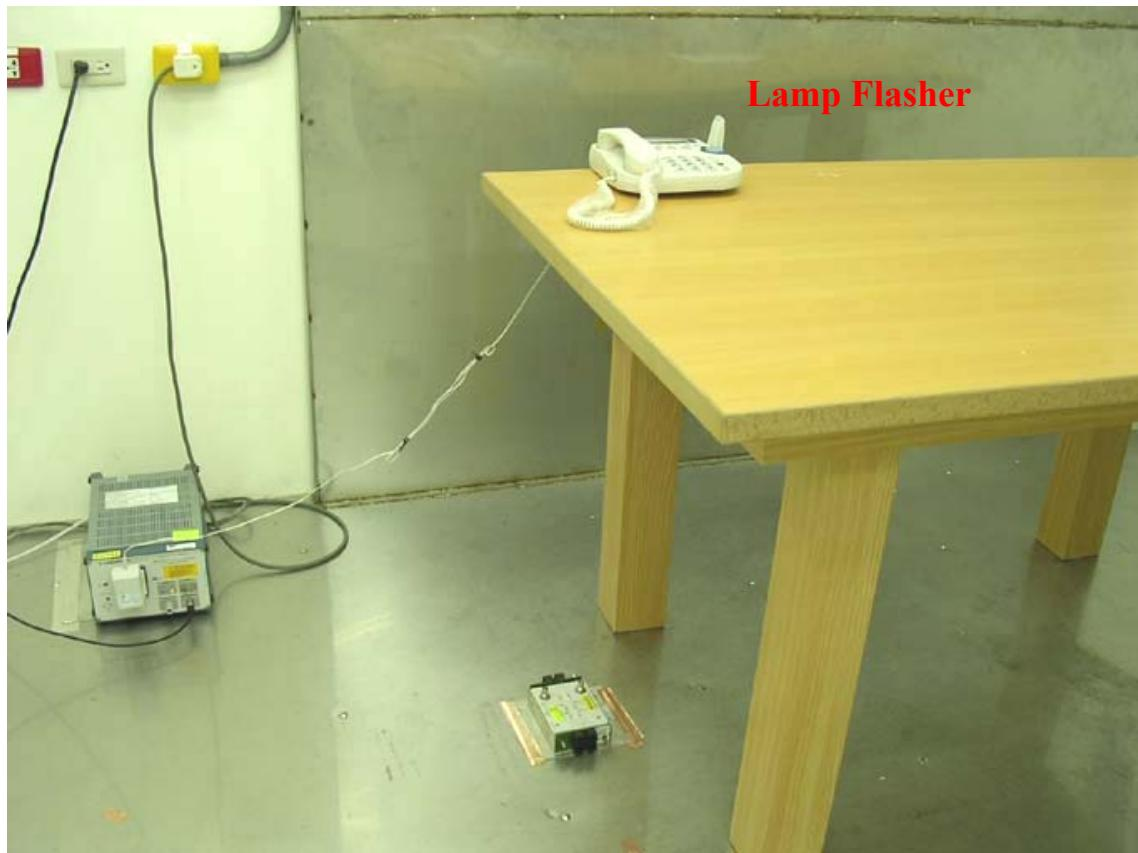
**Photo 2: Conducted Emission Set-up Photo**
