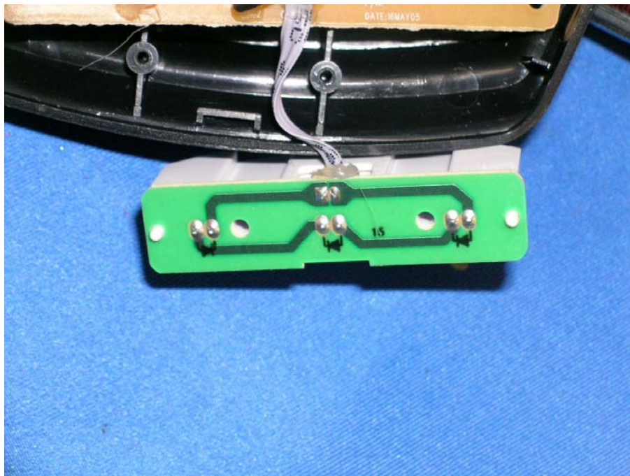
Base Charging Contacts rear side
