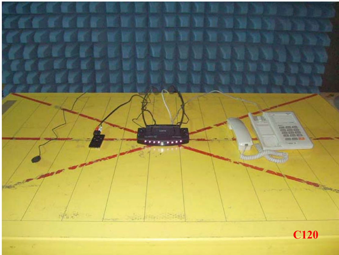
Photo 1: Radiated Emission Test set-up photo
