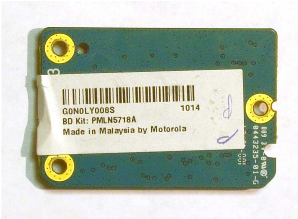
FRONT VIEW OF BLUETOOTH/GPS BOARD
