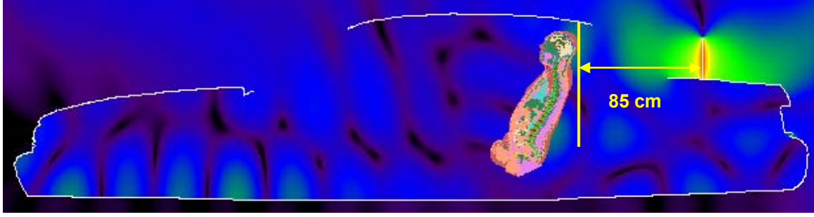
Figure 2: Passenger model exposed to a trunk-mount antenna operating: H-field distribution. The antenna is mounted at 85 cm from the passenger.
