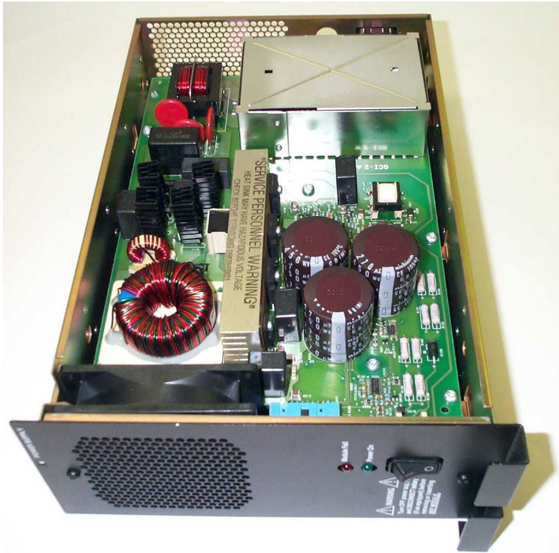
Power Supply Module, Cover Removed
