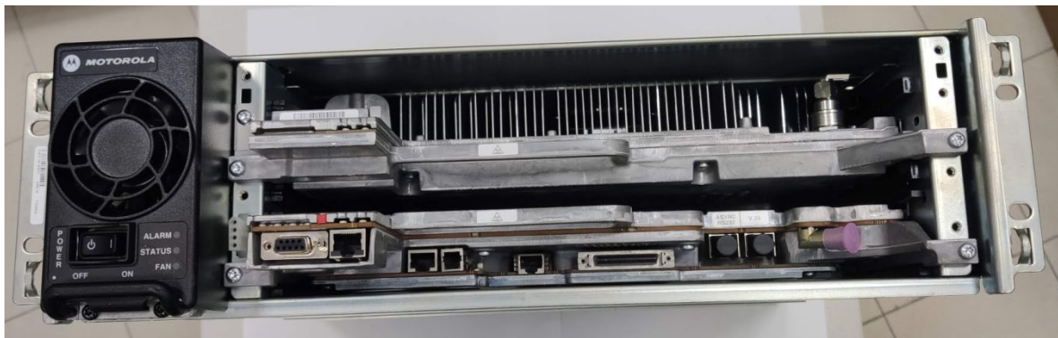
Front View of Base Radio Showing Transceiver Module with TOC Installed and Identifying Connections
