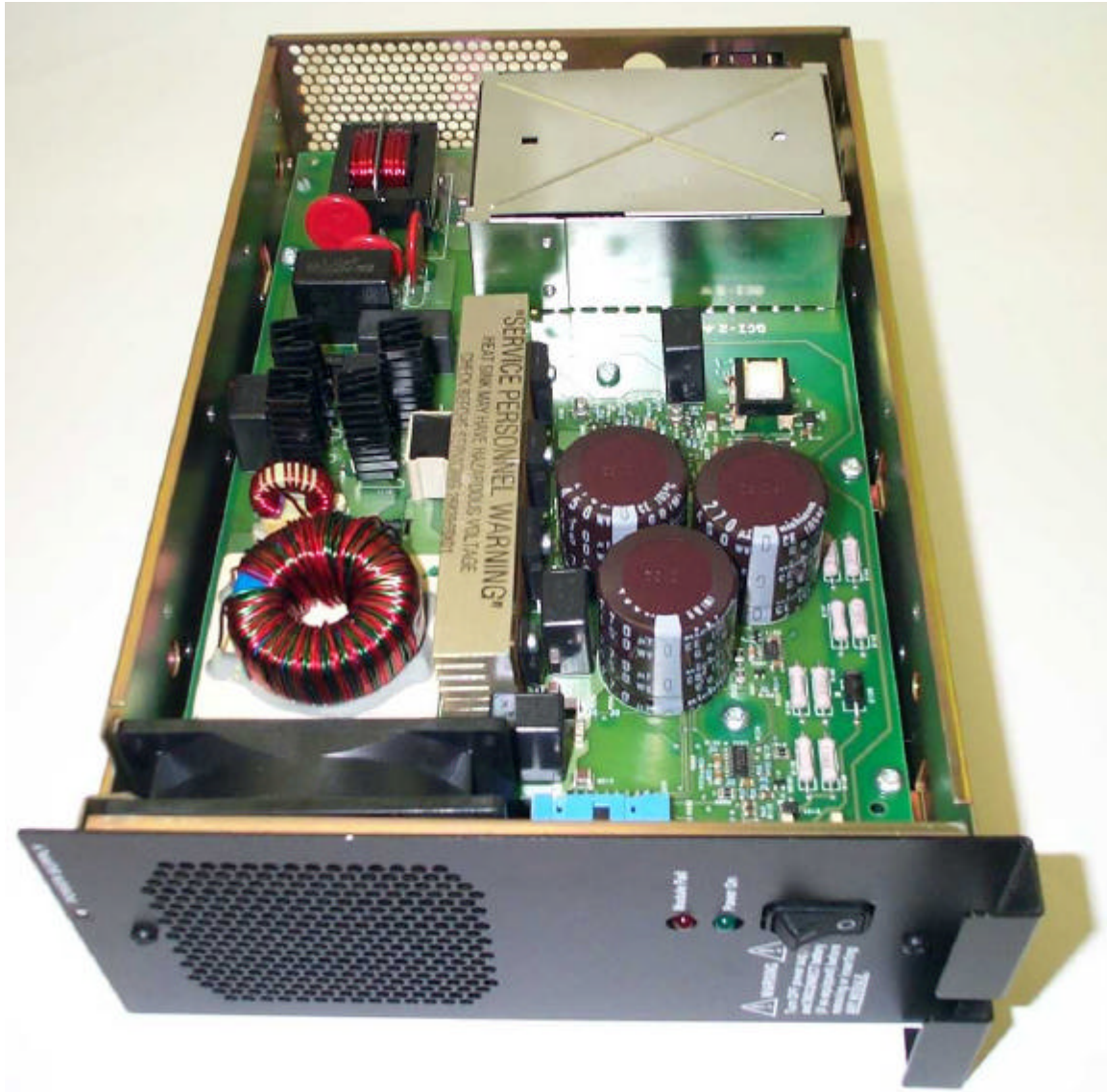
Power Supply Module, Cover Removed
