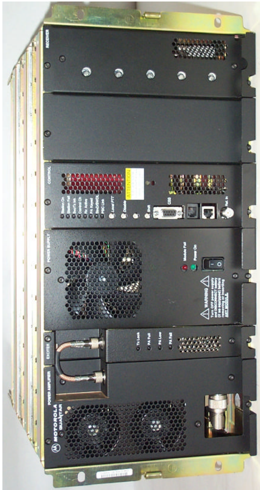
Base Radio -- Front View
