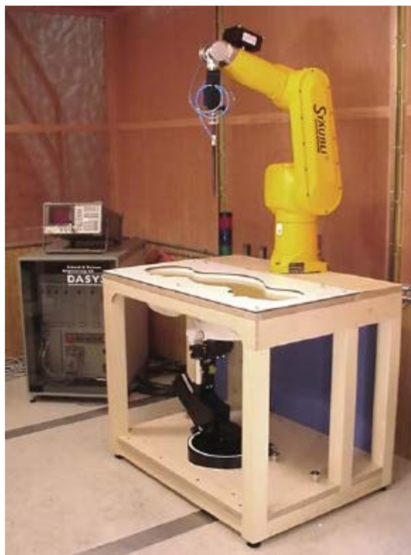
DASY3 SAR Measurement System with SAM phantom
