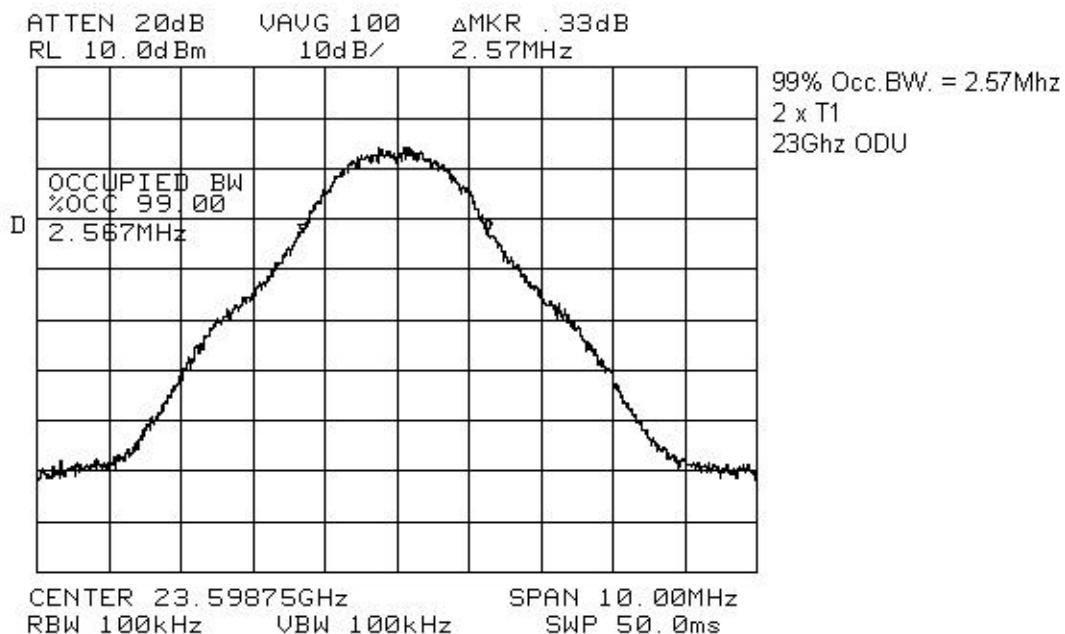
*EQUIPMENT: Digital Microwave Radio, 23 GHz ODU*
