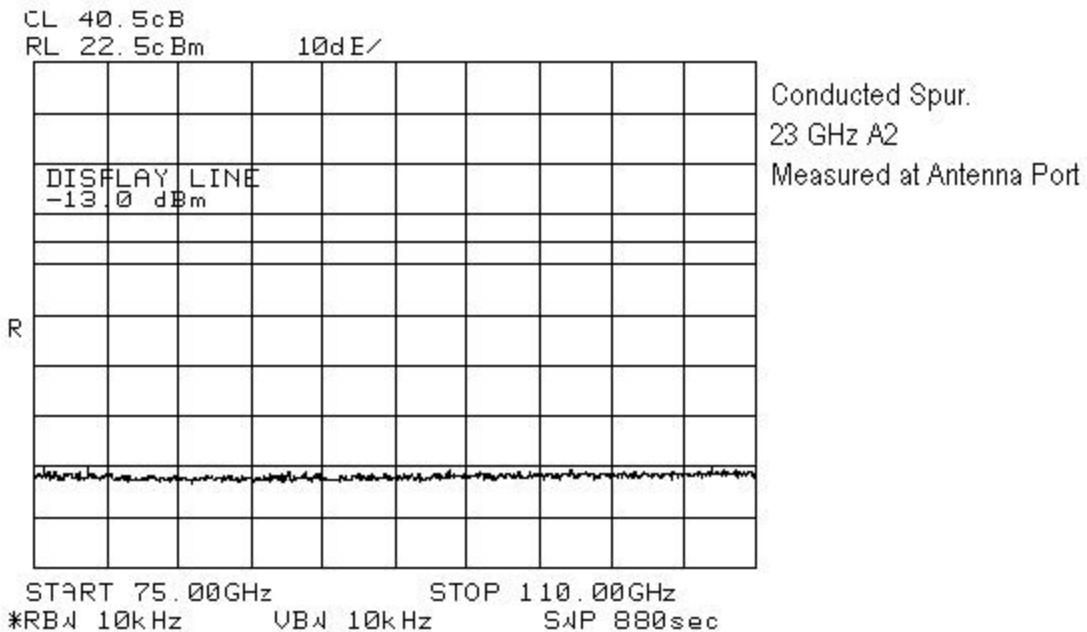
**Section 6. Field Strength of Spurious Emissions****Para. No.: 2.1053****Test Performed By:** Glen Westwell**Date of Test:** October 5, 2000**Minimum Standard:** 101.111 (a)(2)(iii) -13 dBm84.4 dB $\mu$ V/m @ 3m < 1 GHz
