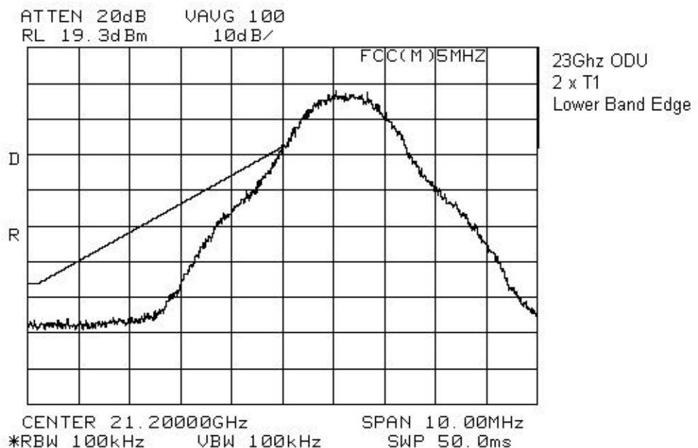
**Section 5. Spurious Emissions at Antenna Terminals****Para. No.: 2.1051****Test Performed By:** Glen Westwell**Date of Test:** October 23, 2000**Minimum Standard:** 101.111 (a)(2)(iii) -13 dBm**Test Results:** Complies.
