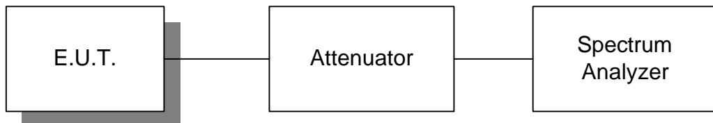
**Para. No. 2.1051 - Spurious Emissions at Antenna Terminals**
