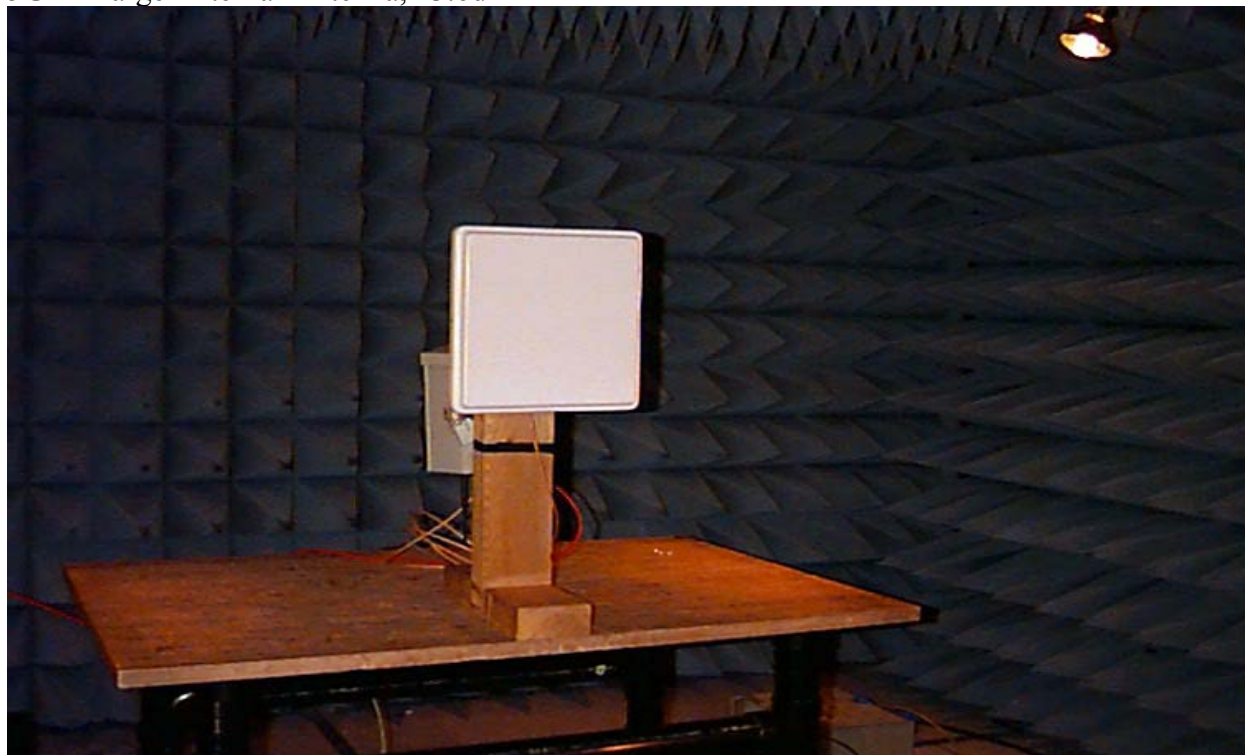
5GHz Large External Antenna, 23.6dBi
