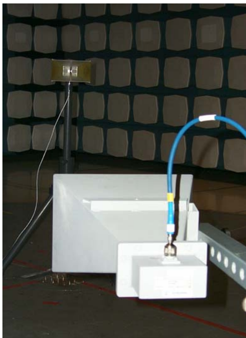
Picture 9: Signal Substitution measurement setup at 3M
