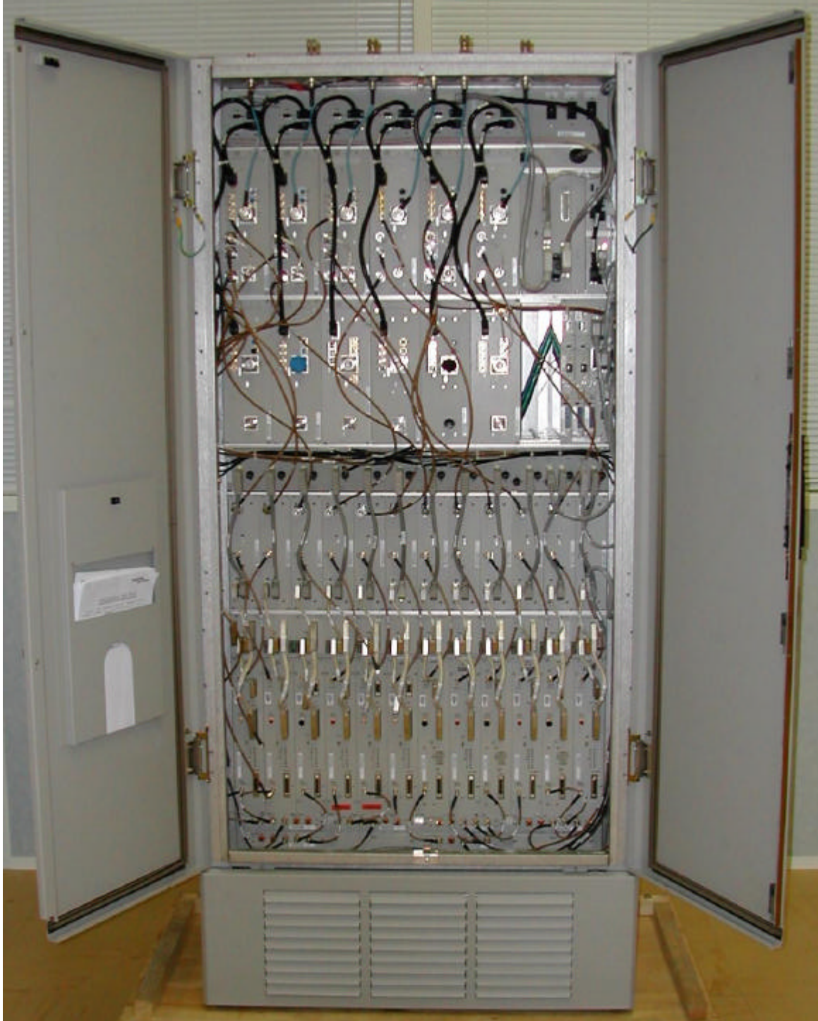
Figure 1: Circuit Boards Mounted in the S12000 Indoor Enclosure
