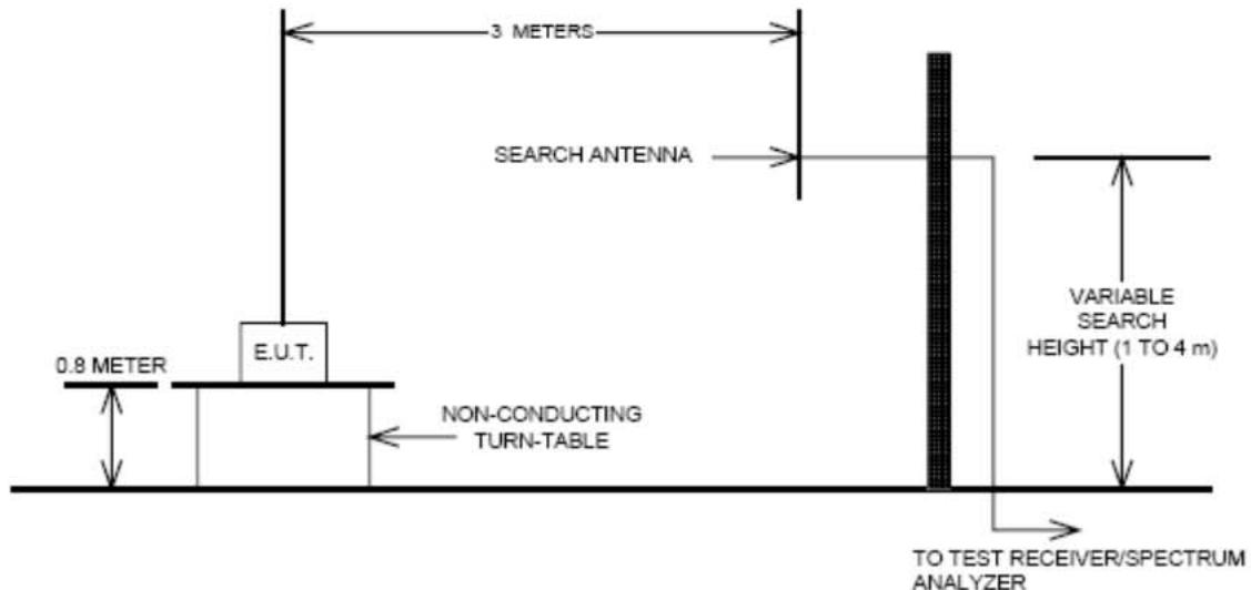
The measurement facilities used for this test have been documented in previous filings with the commission pursuant to section § 2.948. The open field test site is situated in open field with ground screen whose site attenuation characteristics meet ANSI C63.4 –2003. A mast capable of lifting the receiving antenna from a height of one to four meters is used together with a rotatable wooden platform mounted at three from the antenna mast.
