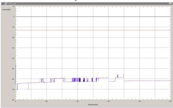
Test: 22.3; Frequency Band = FDD5, Mode = W-CDMA, Channel = 4233, Frequency = 846.6MHz
