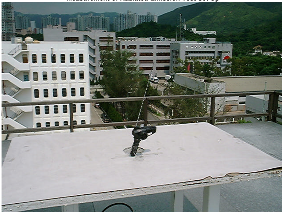
Measurement of Radiated Emission Test Set Up
