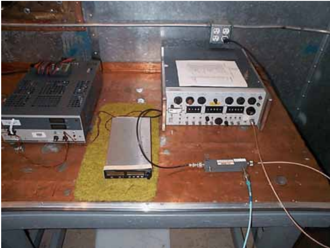
Figure 6-1 Photograph of Occupied of Bandwidth Setup
