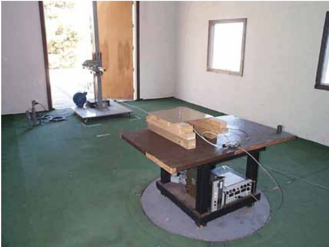
Figure 8-3 Photograph of Field Strength of Spurious Radiation Setup 200 MHz to 1000 MHz Vertical Polarization
