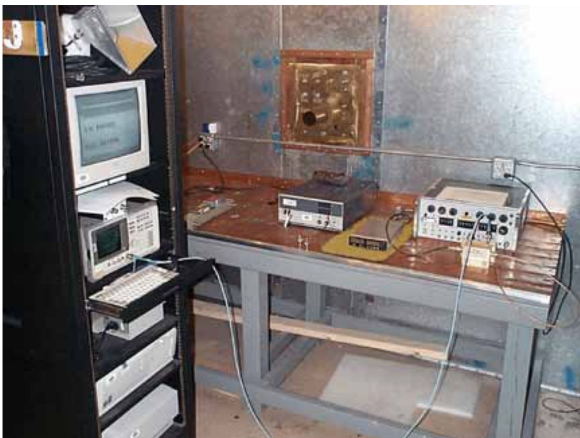
Figure 7-1 Photograph of Spurious Emissions Setup 10 kHz to 200 MHz
