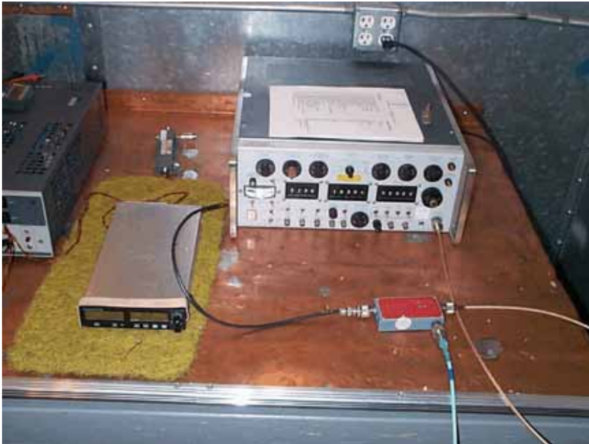
Figure 7-3 Photograph of Spurious Emissions Setup 1 GHz to 2 GHz
