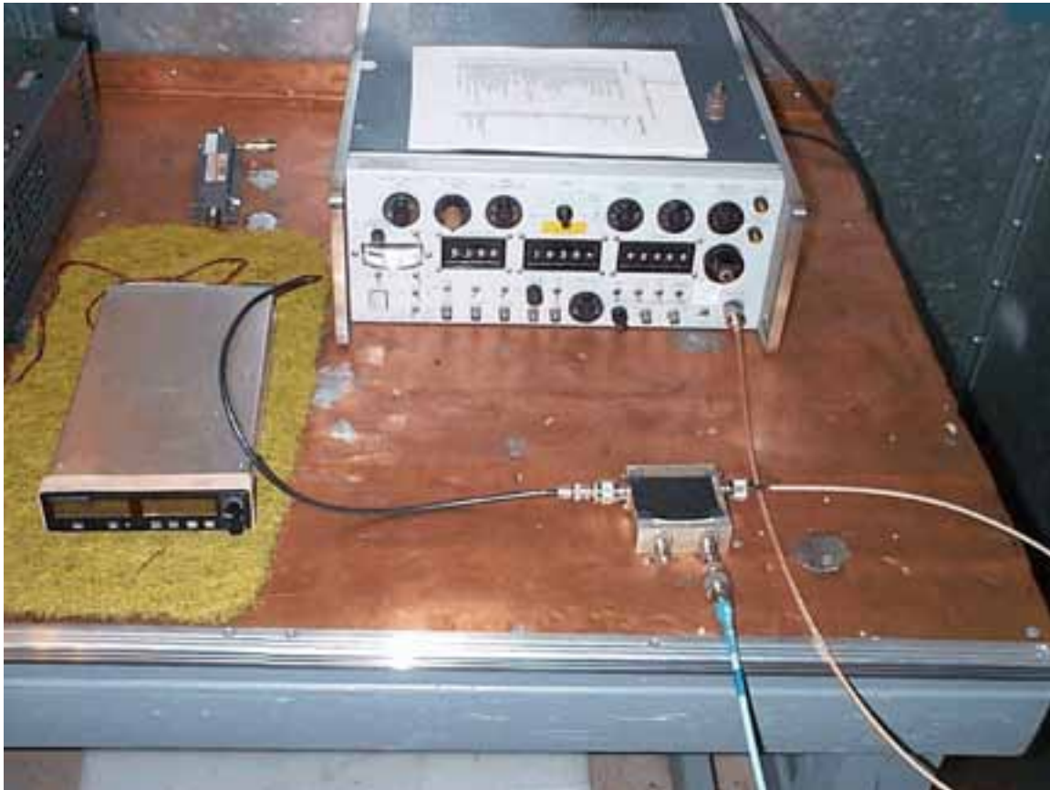
Figure 7-2 Photograph of Spurious Emissions Setup 200 MHz to 1 GHz
