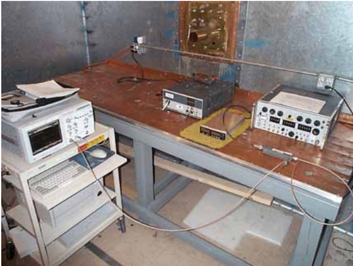
Figure 5-2 Photograph of Modulation Characteristics Setup
