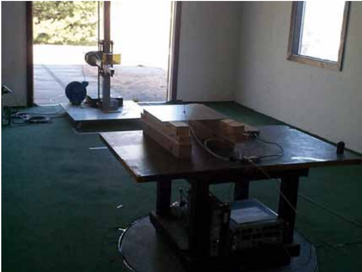
Figure 8-5 Photograph of Field Strength of Spurious Radiation Setup 1 GHz to 11 GHz Vertical Polarization
