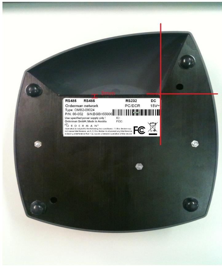
The type-label has a defined position on the bottom side of the OMB2 (picture above)
