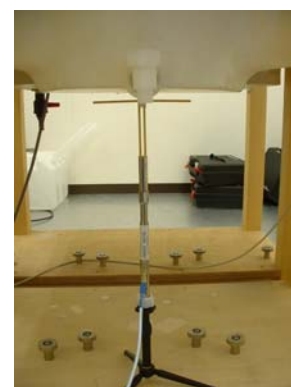
900MHz System performance check setup
