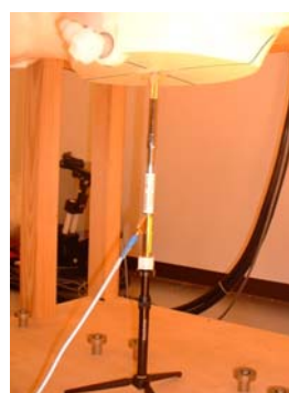
2450MHz System performance check setup
