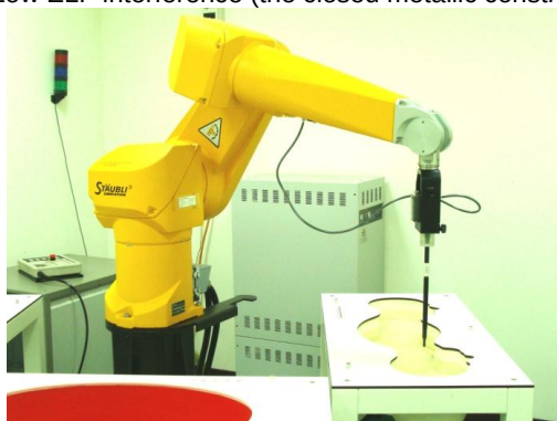
Fig 5.5 Photo of DASY4
