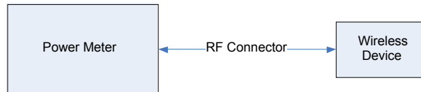
Figure 12-1 Power Measurement Setup
